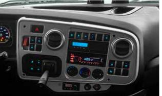
Improved air conditioning system, offered as standard, maintains ideal cabin temperature in all weather conditions.
