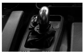
12-speed automated transmission is provided as an option for 420 PS vehicles. The system automatically selects the most appropriate gear for each situation and provides great comfort.
