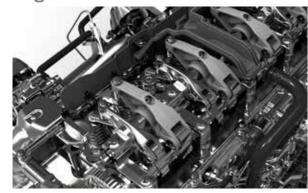
The new integrated engine brake, available as standard equipment, provides additional 320 kW brake power for 420 PS vehicles and 220 kW for 330 PS vehicles. This high brake power can be applied gradually, meeting varying braking needs according to load conditions.
