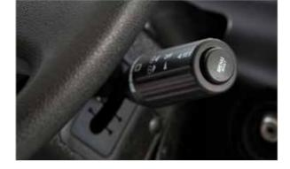
The 600 KW Intarder, which is available as an optional feature on 420 PS vehicles, meets all expectations under such challenging conditions as going downhill while loaded. Preventing unnecessary use of your service brake, it prolongs service life.
