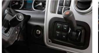
Eco. Off-Road and Rocking modes are compatible with all types of road and terrain. Eco mode provides fuel economy without compromising performance. Off-Road mode is ideal for rough terrain with its excellent traction. And Rocking mode is a powerful support against the risk of getting stuck in muddy terrain.
